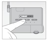
**10.** Hold center button on AP1 camera unit for 5 seconds. Release button, and wait 3 seconds for blinking orange light.
