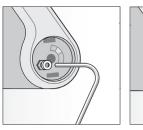
**17.** Tighten the camera angle lock screw, and attach the cover.
