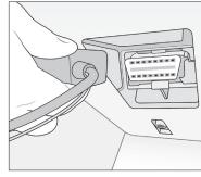
9. Plug main cable into your vehicle's OBDII port. Turn on vehicle. LED sequence will begin. Look for all 3 solid LEDs.
